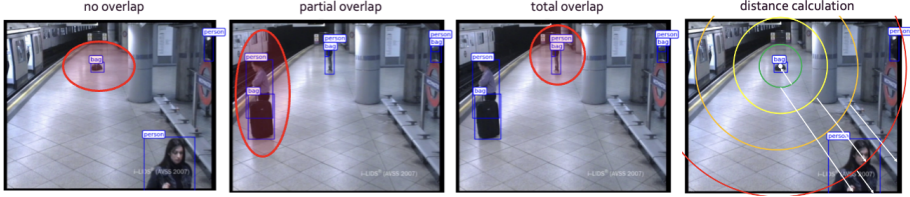
Figure 5. Overlap types and distance calculation for a selected bag [MBT25]. The distance between two objects is estimated as the distance between the centers of their bounding boxes while considering the estimated depth of each object, i.e., a 3-dimensional Euclidean distance is calculated. The calculated distances are binned into five overlapping ranges formed by increasing the radius of concentric circles with the bag of interest in their center.
