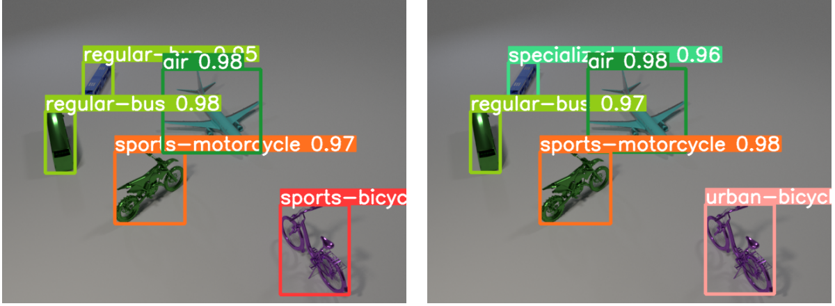
Fig. 5. The left figure shows a scene, based on VT\mathcal{H}4 , in which vehicles corresponding to the “utility bike” and “articulated bus” rare slices are misclassified by YOLOv5 into the “sports bicycle” and “regular bus” classes, respectively. In contrast, the right figure shows the same scene in which such vehicles are correctly classified, after model mending, into their “urban bicycle” and “specialized bus” classes, respectively.
