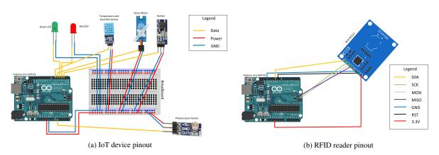
Fig. 5. Physical connections between the Arduino UNO WIFI and the IoT devices used in the Smart House scenario.
