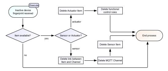
Fig. 7. Item deletion pipeline of the OpenHAB controller.
